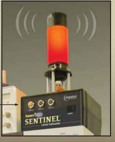
The Beacon illuminates **red** and an audio alert sounds when a level has been reached (full or empty, depending on setup)
