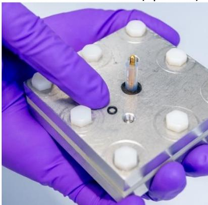
12) Assembled cell. Screw the inlet and outlet tubing connections. In an undivided cell, the fluidic connections in the other end plate can be closed with plugs
