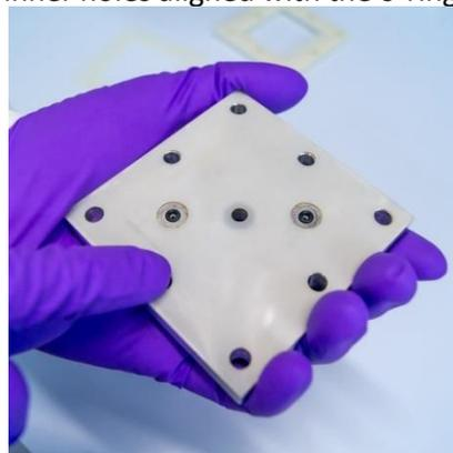
3) Add an alignment gasket for the cathode
