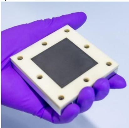
8) Add an isolation layer (this layer also has inner holes, in case an undivided cell needs to be assembled)
