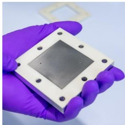
5) Add the electrode separator/reaction channel foil
