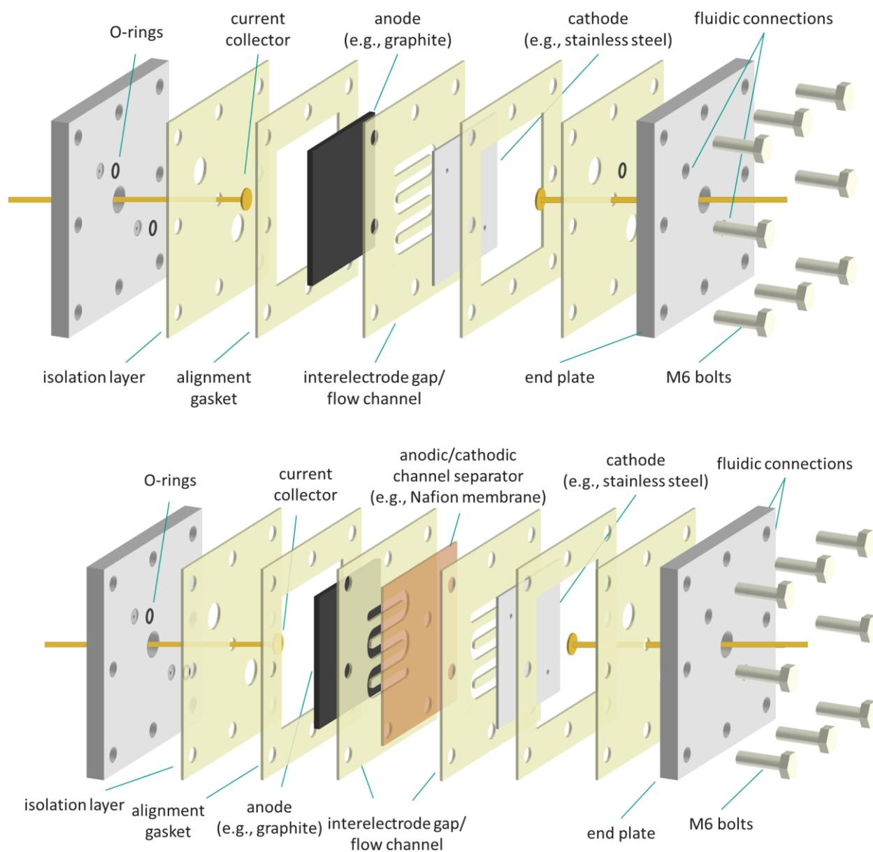
**Figure S1.** Exploded view of the assembly of an undivided cell (top) and a divided cell (bottom).
