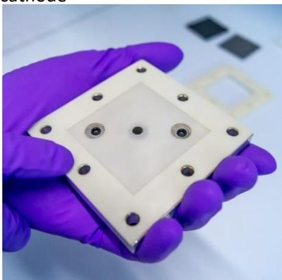
4) Add the cathode. Check the alignment of the electrode holes and the o-rings
