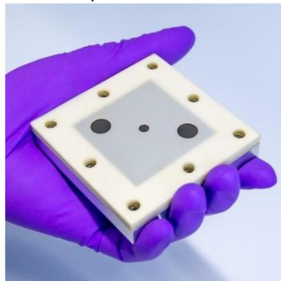
9) Place the second end plate and screw the bolts. This end plate also has fluidic connections, so the setup can be used as a divided cell
