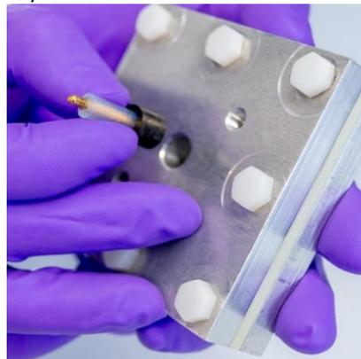
11) Introduce o-rings (5x3 mm) in the fluidic connections (optional)
