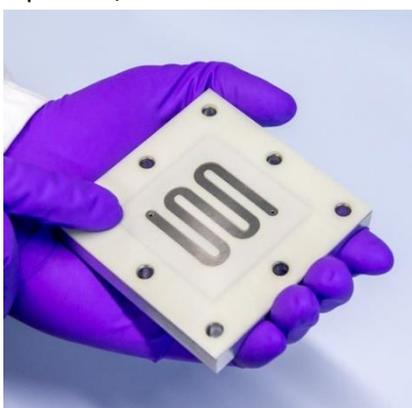
6) Add alignment gaskets. The total thickness should be similar to the electrode thickness. In this case, 10x0.3 mm gaskets were used for a 3 mm thick anode
