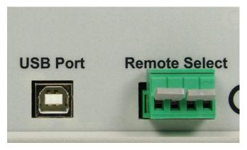
pump, etc. Attach leads to the supplied Green plug. Once contact is established at the other end of the leads, the controller will automatically disengage or engage heating values.
