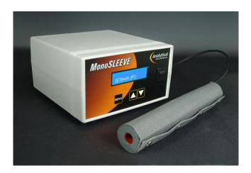
The MONOSLEEVE controller is designed for use in analytical format liquid chromatography applications only.
