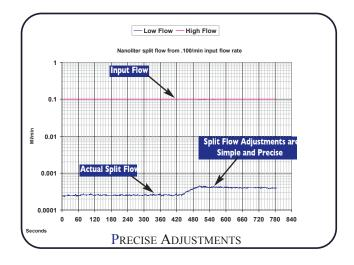
**Model 63 Binary Fixed Splitter** with its interchangeable fluid resistors, eliminates the need to cut capillary tubing to change the split ratio. Split ratios can be changed by replacing the resistor set.
