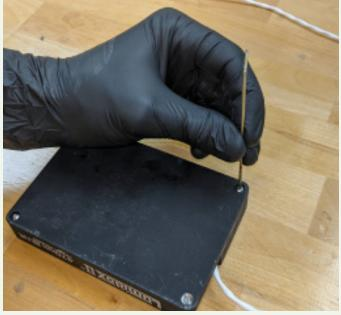
STEP 2: Using the same 1/16" Allen key, secure the bottom plate of the Lumidox II with the 4 shorter screws.
