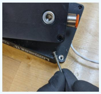
**NOTE:** Ensure that the screw with the washer is used for the shallow hole near the cable exit location.
