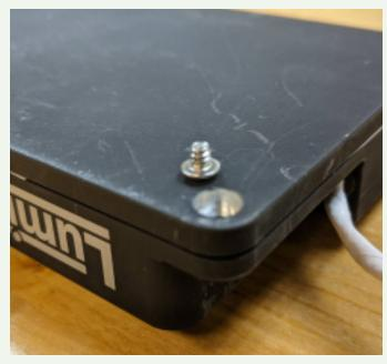
NOTE: Ensure that the shortest screw is used for the shallow hole near the cable exit location.
