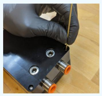
**STEP 2:** Place the Thermal Transfer Deck on top of the array, and secure it using the 4 longer screws (provided), using the same 1/16" Allen key.
