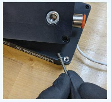
**NOTE:** Ensure that the screw with the washer is used for the shallow hole near the cable exit location.
