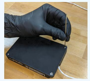
**STEP 1:** Turn the Lumidox II LED array over, and using a 1/16" Allen key, remove the 4 screws securing the bottom plate.
