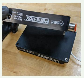
**STEP 1:** Turn the Lumidox II LED array with the Thermal Transfer Deck over, and using a 1/16" Allen key, remove the 4 screws securing them together. Gently lift the TTD away.
