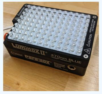
**STEP 3:** Turn the Lumidox II array / Thermal Transfer Deck over. The product is now ready for use.
