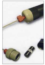
Moisten the free end of the cartridge and reassemble the Holder. Tighten the Holder Ends by hand until they are snug. **Do Not Use Wrenches or Pliers!** The PEEK cartridge end pieces are interchangeable. The knurled end of the aluminum body facilitates opening and closing the Holder and can be used as a flow direction reference after a cartridge is placed in the Holder.
