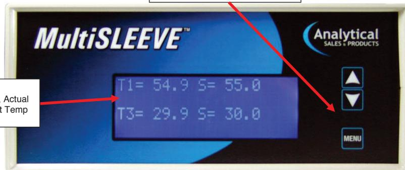
Turn the Column Heater on. The temperature controller will perform a self-diagnostic test upon power-up. If, after powering up, the display indicates something other than reasonable temperature values, notify Customer Service for further action.
