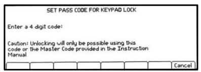
The pass code is a "once only" code. After the system has been unlocked, the pass code is discarded and a new code (or the same one) must be entered in order to lock it again.
