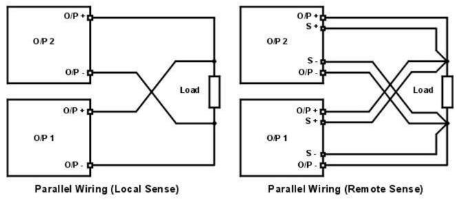
The drawing shows a parallel connection of two outputs using local or remote sensing.
