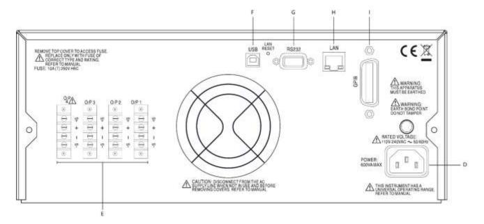
D- The MX100Q has only an AC power connection socket on the rear panel.
