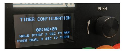
To enable the countdown timer, select the menu by pressing the center control knob ("PUSH") once while on the home screen. Follow the on-screen directions to configure time. Press and hold *START/CANCEL* for 2 seconds to arm. **Ensure safety goggles and shields are in place**. Press *START/CANCEL* again to illuminate. Remaining time is displayed in the upper right of the screen.
