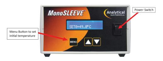
Turn the Column Heater on. The temperature controller will perform a self-diagnostic test upon power-up. If, after powering up, the display indicates something other than reasonable temperature values, notify Customer Service for further action.
