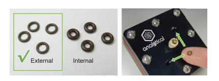
**5.** Insert the external o-rings (F1088302) into the deep diagonally positioned holes in the Lid and Base End Plates. These are where the fluid connections will be made.
