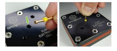
**2.** With the flow electrolysis cell fully assembled, gently place the pogo pin / ferrule assembly into the center hole of the end plate. Ensure that the spiked head of the pogo has is making contact with the electrode.
