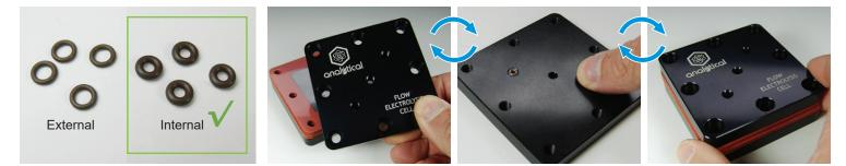
**12.** Find the Lid End Plate. Insert two internal o-rings (F1088301) into the shallow unthreaded diagonal holes (in the side of the plate opposite the logo engraving). Place the Lid End Plate with o-rings on top of the assembled stack, making sure that flow holes are lined up.
