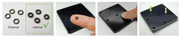
**2.** Insert two internal o-rings (F1088301) into the shallow non-threaded diagonally positioned holes.
