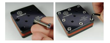
**10.** Insert 8 M6 screws through the holes of the lid plate and the layers beneath it, then screw them into the bottom plate with an alan wrench.
