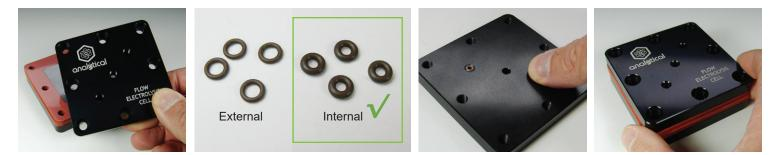
**9.** Find the Lid Plate. Insert two internal o-rings (F1088301) into the shallow unthreaded diagonal holes (in the side of the plate opposite the logo engraving). Place the Lid Plate with o-rings on top of the assembled stack, making sure that flow holes are lined up. **Tip:** use your thumb or finger to press the o-rings into the holes. This will help keep them in place when placing the lid plate onto the assembly.
