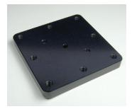
**1.** Place the Base Plate (black aluminum with *threaded* holes) on a flat working surface. Make sure that the side with the shallow diagonally positioned holes are facing up.
