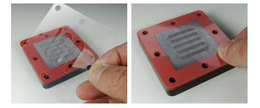
**8.** Place the second flow channel film (from set of 2) on top of the ion exchange film.
