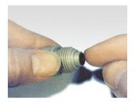
To replace a filter, disassemble the holder and remove the old unit with a fingernail or tip of a spatula. Inspect both sections of the Holder for buffer salt crystals or other debris. Rinse and dry if necessary before inserting a new filter element.
