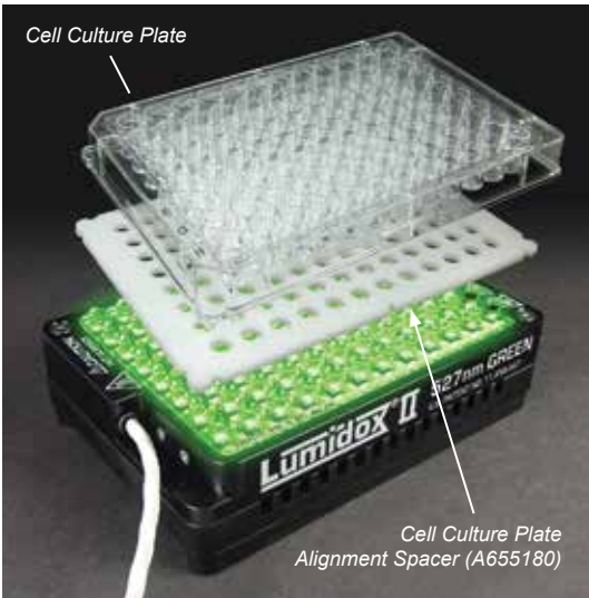
Lumidox / Cell Culture Setup
