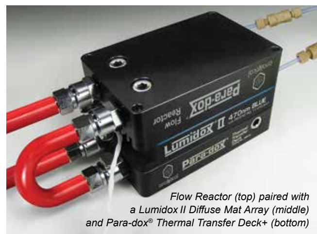
Lumidox II Diffuse Mat Array placement
