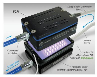
**Typical configuration:** 48-position TCR used in conjunction with a Lumidox®II 48-position **Solid Base** LED Array, a "Straight-Thru" Thermal Transfer Deck (for additional cooling of array) and connected to an external liquid chiller.
