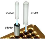
Both the 24-well and 96-well blocks will hold 750µL, 8 x 30mm flat bottom glass inserts (part no. 84001). They will also hold 250µL, 5 x 31mm inserts (part no. 20303) when used with anodized aluminum spacers (part no. 96969).
