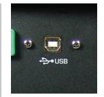
USB Used to initiate / first connection of ModBus RS-485 chain
