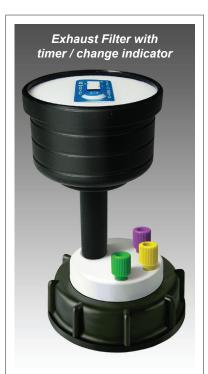
Canary-Safe waste caps use an **exhaust** *filter* which contains an activated carbon material that absorbs 99% of all vapor and particulate materials evaporating from your solvents.
